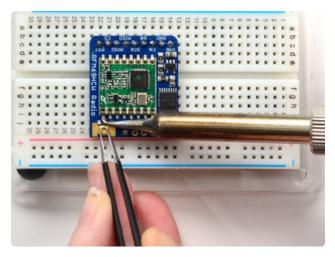
Solder in the first pad while holding the uFL steady
