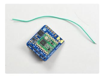
Cut a stranded or solid core wire the the proper length for the module/frequency
