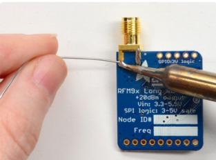
Flip over and also do the other side ground/mechanical contacts
