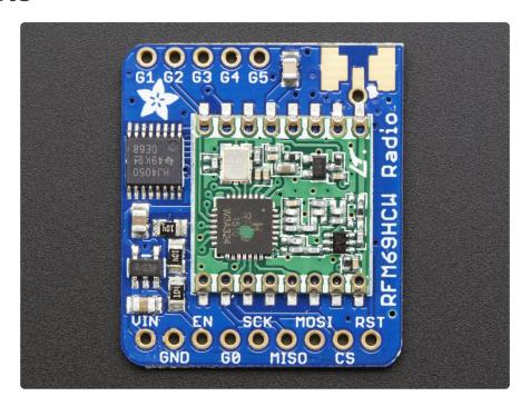
Both RFM69 and RFM9x LoRa breakouts have the exact same pinouts. The silkscreen will say RFM69HCW or LoRa depending on which variant you have. If there's a green or blue dot on top of the module, its 900 MHz. If there's a red dot, its 433 MHz
