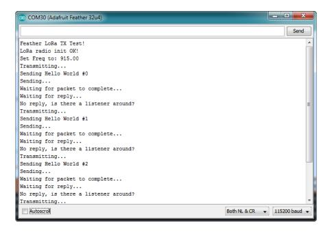
Now open up another instance of the Arduino IDE - this is so you can see the serial console output from the TX Arduino while you set up the RX Arduino.
